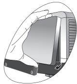
4. Loosen the screws that hold the lamp to the projector. If the screws are not loosened completely, they could injure your fingers. It is strongly recommended that you use a magnetic-head screwdriver to retain the screw should it come loose.
